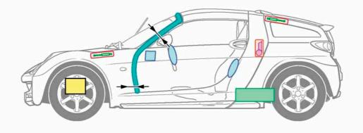
Legend Structural Airbag Battery 0 0 000 000 reinforcements High-voltage Gas generator Rollover protection D /4\ components Seat belt Fuel tank Cutting points tensioner Gas filled Control unit ₽.... spring device
